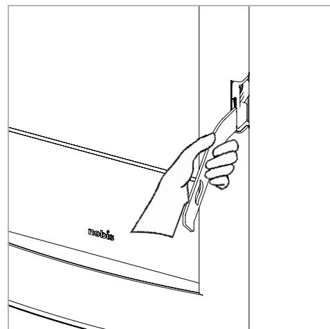
Lift the "cold lever", supplied with the product, to release the door and allow fire door opening, as in the figure below:
