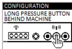
Keep the remote communication key
