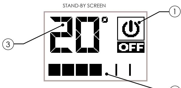
**i** After 20 seconds of inactivity, the display on the handheld device blacks out and passes to "SLEEP" mode, maintaining the remote connection with the appliance. The display re-enables only by pressing the **1** key.
