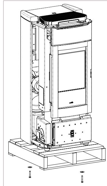
Position the equipment and proceed with its connection to the chimney flue. Find, using the 4 adjustment feet, the right level so that smoke discharge and the pipe are connected correctly.
