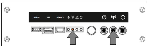
The yellow, flashing led, under the icon
