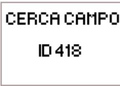
This screen indicates the handheld device is trying to communicate with the appliance, a useful operation to recover information to display to the end user. (1)
