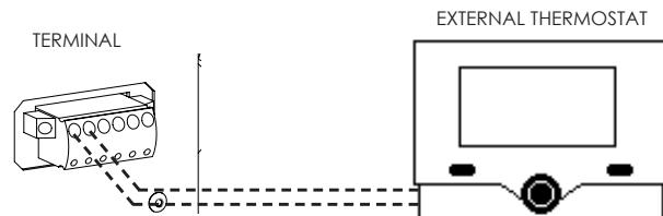
Following electrical connection, to allow the control unit to recognise the presence of the t.text, the recognition function must be enabled from the SETTINGS menu (see the "ENABLE EXTERNAL THERMOSTAT" paragraph)
