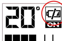
As soon as the level of the batteries does not allow any remote communication, the handheld device displays, on the full screen, the image of the flat battery, blocking all the functions connected to it until the batteries are replaced.
