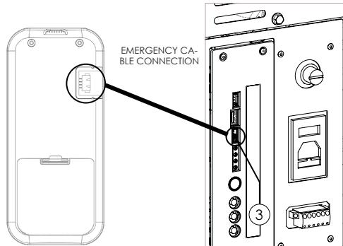
**!** Before connection using the emergency cable, remove the batteries from the handheld device from the specific compartment. **DANGER OF FIRE**
