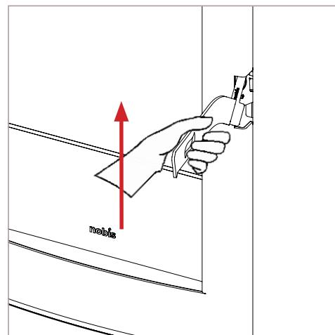
To extract the flame trap, lift it slightly as in the figure below:
