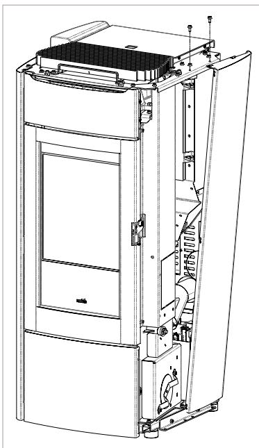
Remove the pre-drilled blank from the sheet metal with the assistance of a suitable tool (e.g. pry with screwdriver)
