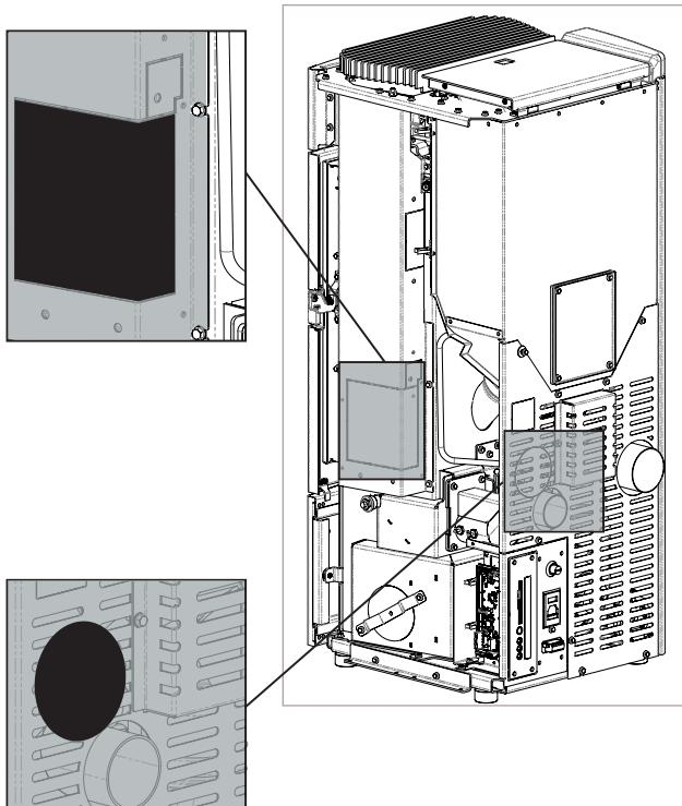
**!** The installation of the ducting, without removing the pre-drilled hole blank, will result in NO heat being emitted from the ducting.
