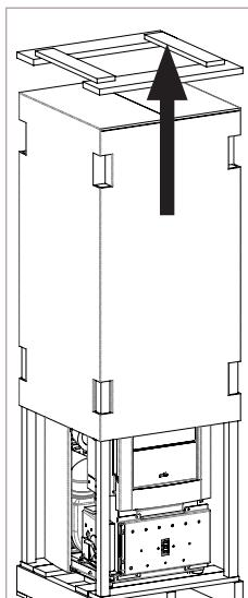
To remove the appliance from the pallet, you can remove the two screws placed under the pallet (13 hex key) to release the appliance from the wooden base.
